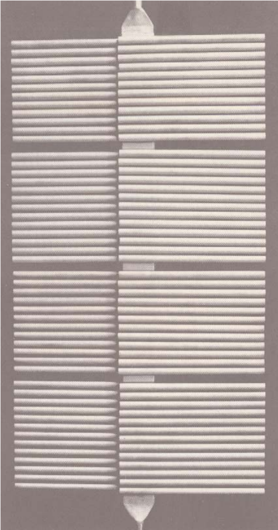
HEAT RADIATOR FOR SPACECRAFT incorporates 100 stainless-steel heat pipes (horizontal tubes) in which the working fluid is sodium. The heat pipes are designed to remove heat from the condenser section of a potassium-filled "loop" (flattened vertical tube), which in turn passes through the nuclear reactor and turbine used to power the spacecraft. The advantages of using heat pipes to dissipate unwanted heat in space include light weight, gravity-free operation and efficient dispersion of heat over a large radiating surface. This particular radiator is designed to dissipate 50,000 watts of heat energy at an operating temperature of 1,420 degrees F. The entire assembly measures 23 inches by 43 inches and weighs only 17 pounds. The device was developed for the Air Force by RCA; one of the horizontal heat pipes was used for the demonstration shown in the color photograph on page 3 .
