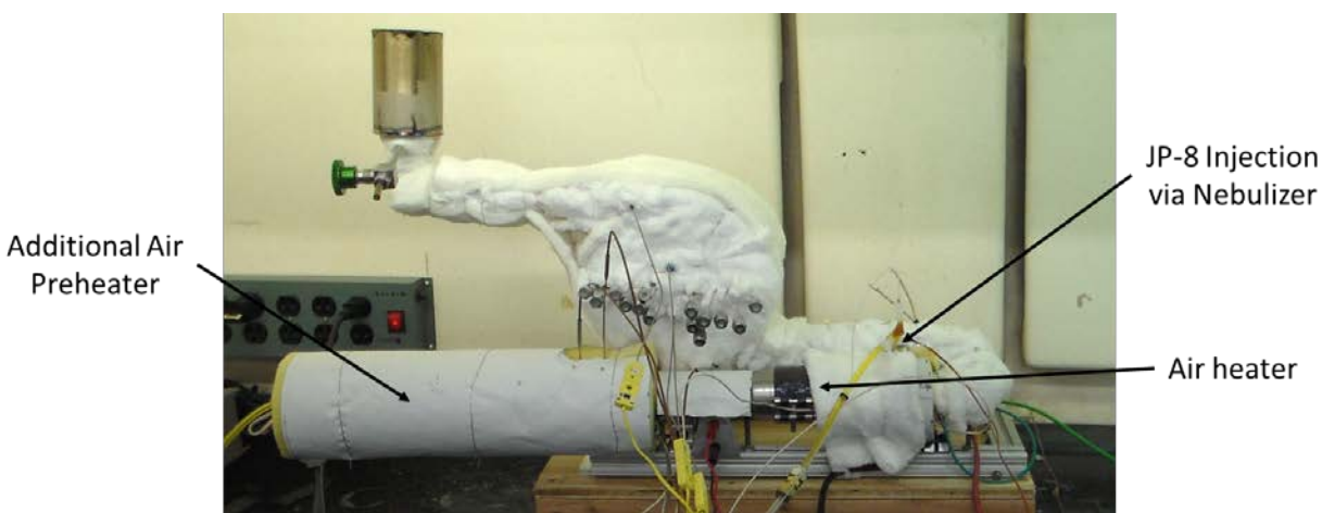
Figure 2: Test setup with air preheater, JP-8 vaporization chamber, Swiss-roll, and exhaust flare.
