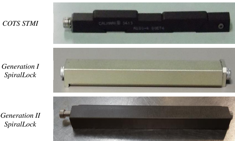
Figure 4. Comparison of COTS STMI, the Generation I SpiralLock, and Generation II SpiralLock STMI Designs.
