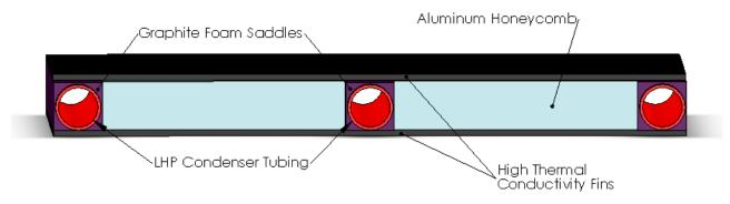
FIGURE 7. Cutaway Section Through a High Temperature Titanium/Water Radiator.
