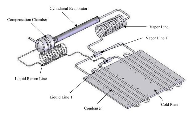
FIGURE 1. Titanium/Water Loop Heat Pipe Layout.
