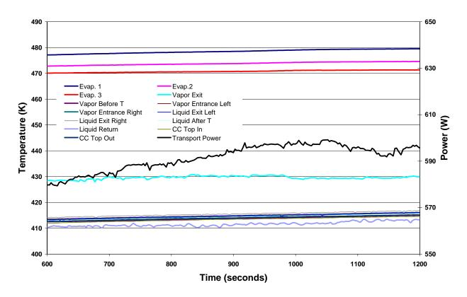
FIGURE 6. Test results from the titanium/water LHP. The LHP carried 590 W at 413 K.
