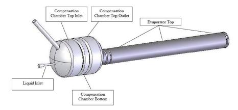
FIGURE 4. Evaporator and compensation chamber thermocouple locations.
